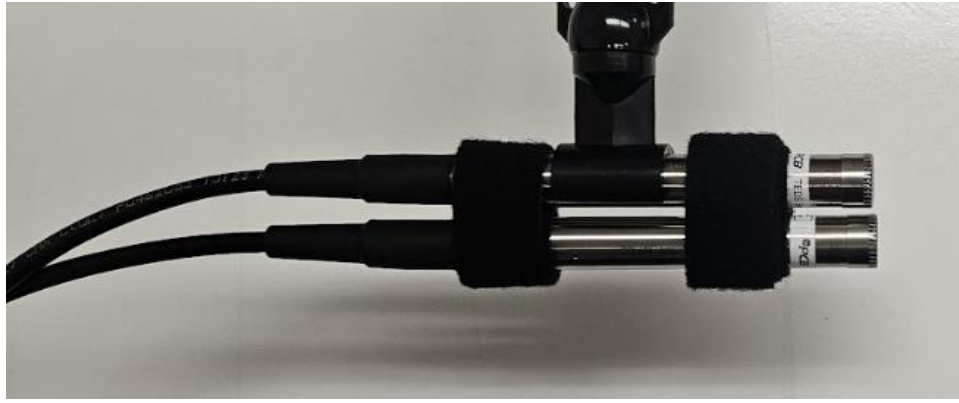
Figure 10: Two electrically isolated PCB 378B02 microphones with unblocked pre-amplifier vents.
