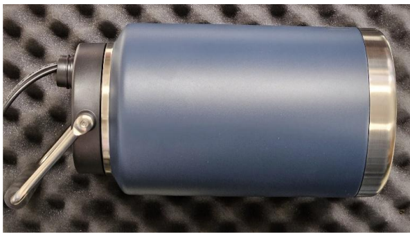
Figure 11: Quiet test chamber with microphone pair mounted in lid (left).
